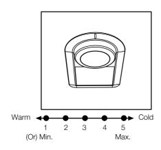
0=System cooling is off. 1=Lowest cooling setting (Warmest setting). 5=Highest cooling setting (Coldest setting).
