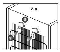
**2. b)** The condenser of your appliance is located on the back as shown below. In order to achieve better energy efficiency with lower energy consumption, please pull the condenser towards yourself as illustrated in picture below.
