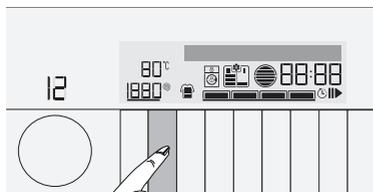
Press the **Spin Speed Adjustment** button to change the spin speed. Spin speed decreases gradually.
