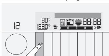
Press the **Temperature Adjustment** button to change the temperature. Temperature will decrease by steps of 10 °C.
